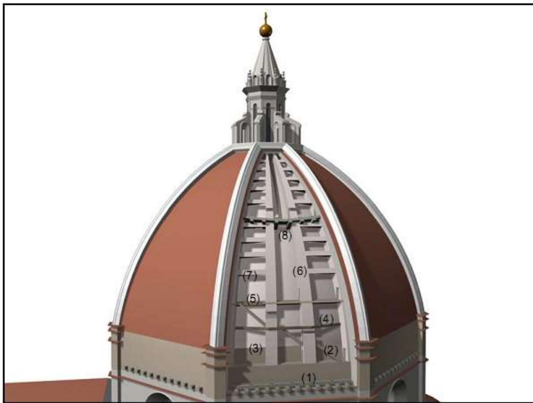
Figure 3. Internal structure of dome: (1) first stone chain, (2) internal walkway within shells, (3) transition from stone to brick masonry, (4) timber ring, (5) second stone chain, (6) vertical rib, (7) horizontal arches, and (8) third stone chain.
