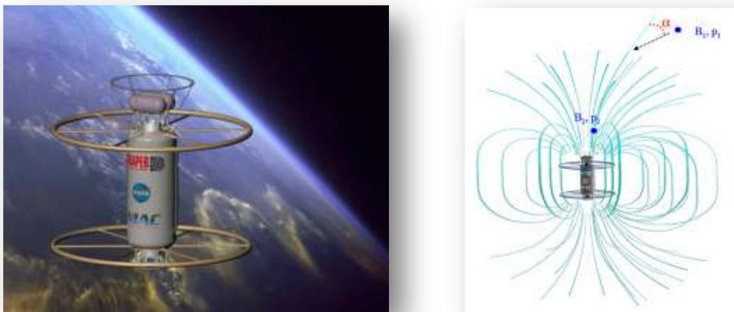
**Figure 7**– Artist concept of the proposed antimatter collection system. This Bussard magnetic scoop is based on the concept of superconducting rings capturing antimatter particle as fuel for interstellar travel. (James Bickford)
