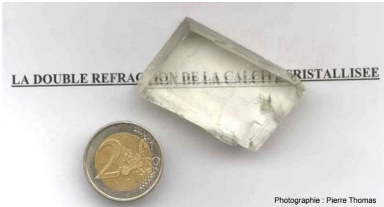
DOUBLE REFRACTION OF ICELAND CALCITE OR ICELAND SPAR
