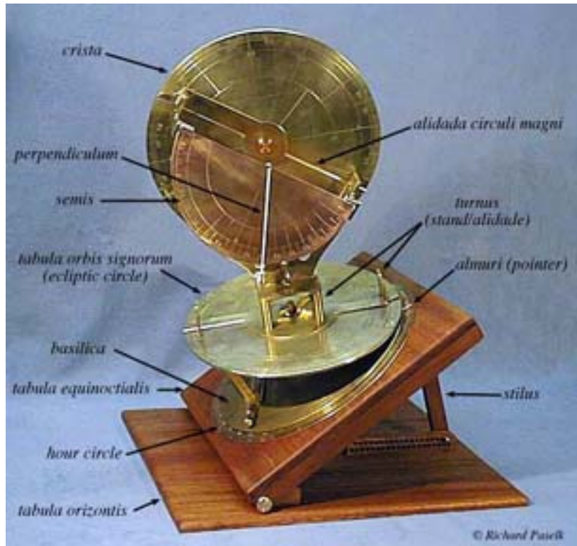
Figure 1. The Torquetum . (The Twisted)
