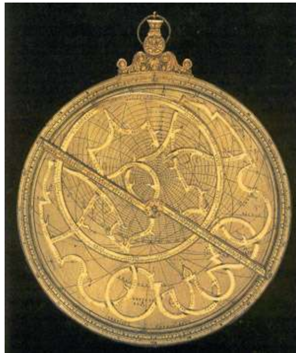
Figure 1. Astrolabe from the 10 th century Abbasid Renaissance showing Table, Rete, and Alidade.
