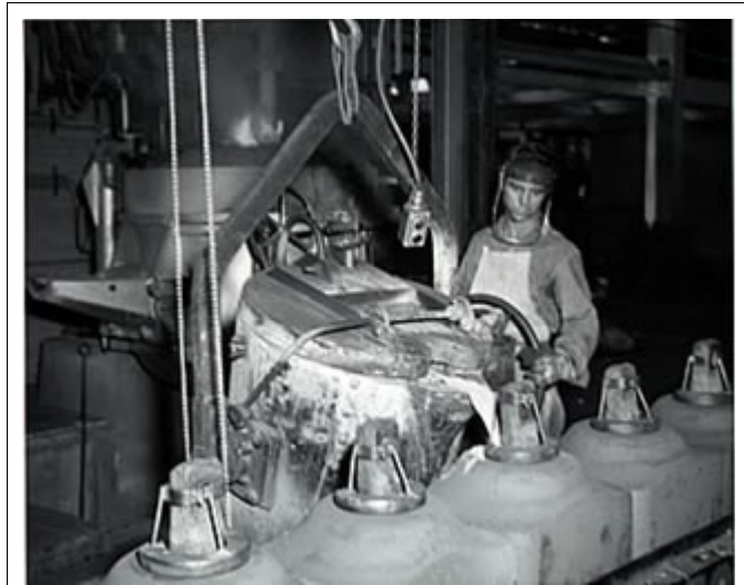
The pouring of molten aluminum around a steel slab in the carbon anodes used in the smelting of aluminum at a plant near Wenatchee
