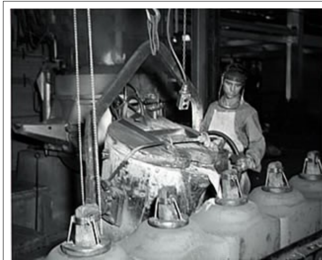
The pouring of molten aluminum around a steel slab in the carbon anodes used in the smelting of aluminum at a plant near Wenatchee
